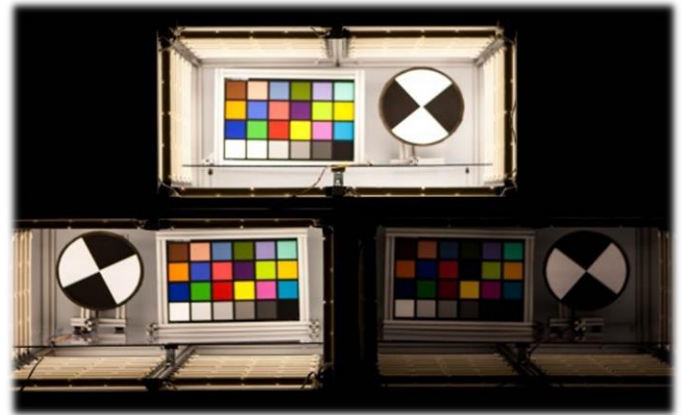
DYNAMIC: 3up HDR test setup, 1 – 180 000 lux
